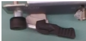
Figure 4-9 Securing Latch - Unlocked and Unlatched
