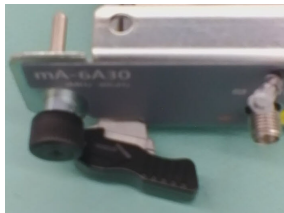
Figure 4-7 Securing Latch - Locked Position
