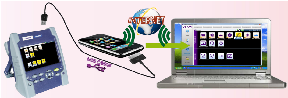
Figure 45 USB connection through Smartphone
