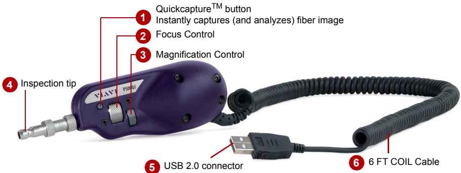
Figure 14 P5000i Probe components
